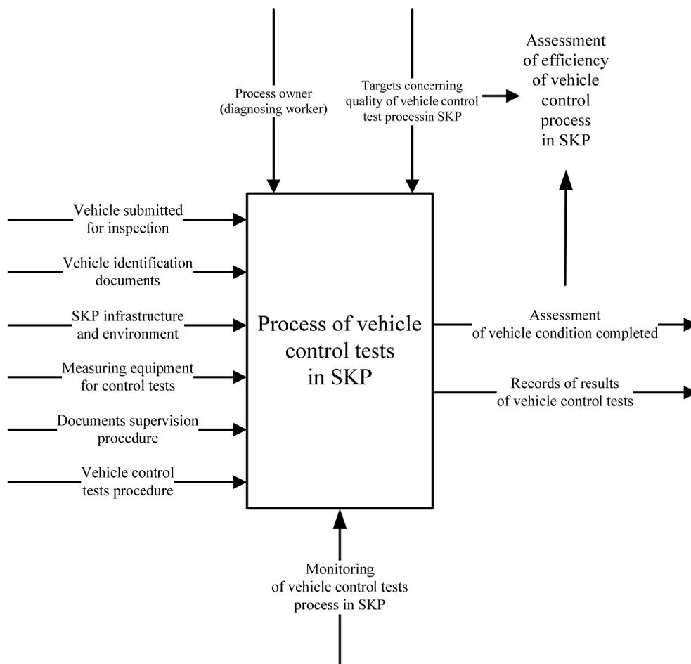
Fig. 3. Quality characteristics the vehicle inspections process at the SKP. Source: own papers
