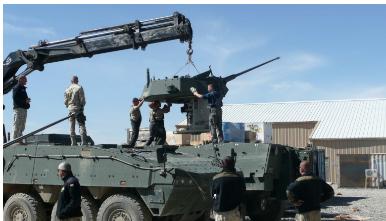
Fig. 1. Maintenance of Armored Infantry Vehicle “Rosomak” during operation ISAF Source: photo of S. Budek
