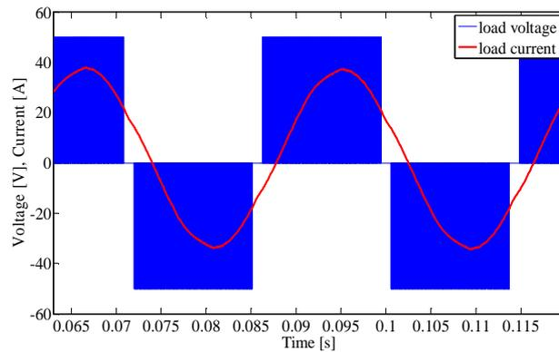
Fig.6. Matrix converter output voltage and current without LC filter with motor load (current waveform was fitted to the picture)
