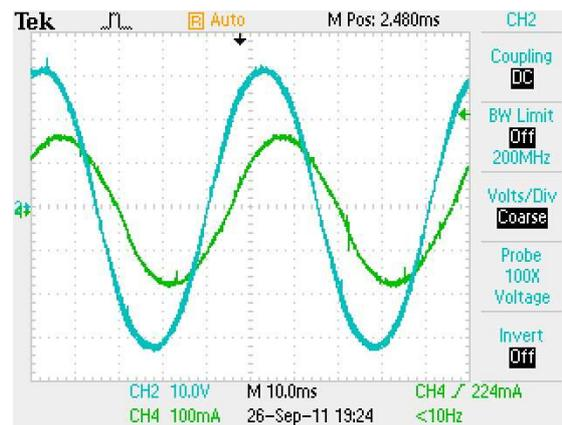
Fig.12. Output voltage (blue) and current (green) of two-stage converter with LC filter and motor load
