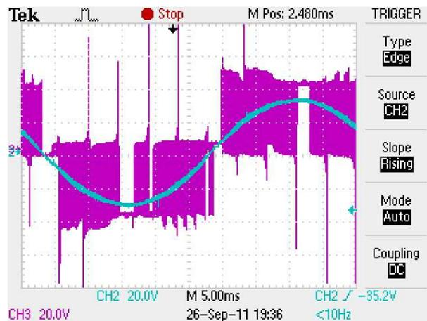
Fig.10. Input (magenta) and output (blue) voltage of LC filter
