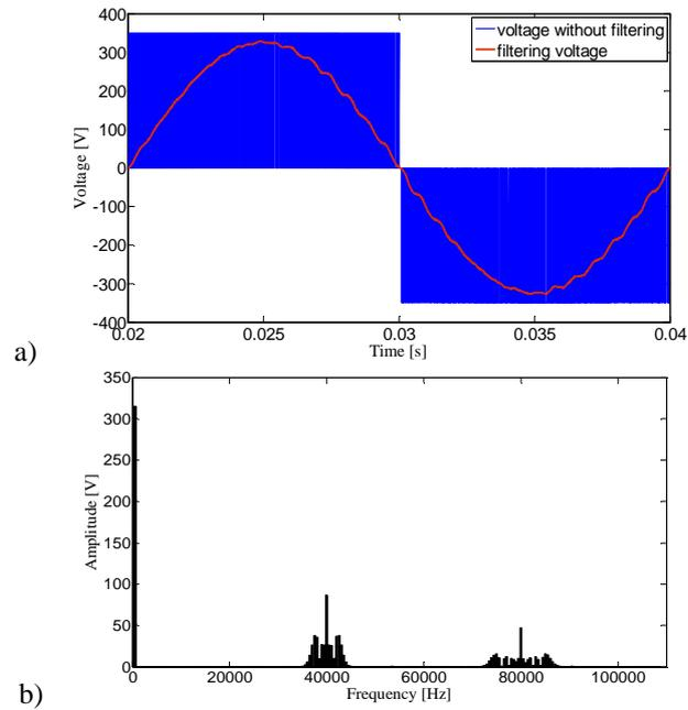
Fig.4. The output voltage of the 1-phase inverter under bipolar PWM control (a) and its harmonic content without filtering (b)
