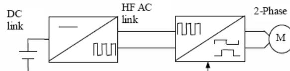
Fig.1. Principle block diagram of 2-stage DC/AC/AC converter (without HF transformer)
