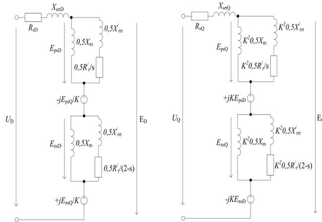
Fig.3. Equivalent circuit of TPIM
