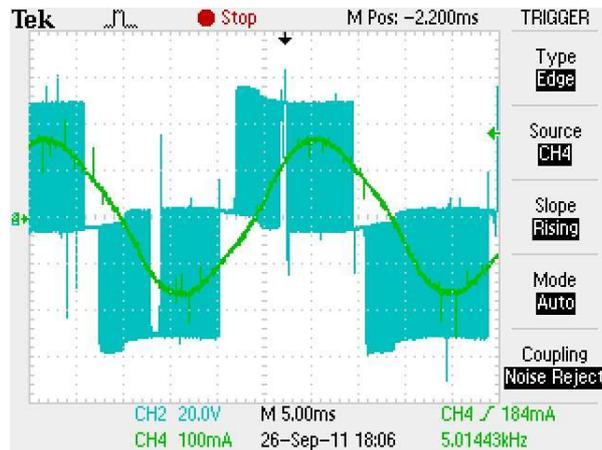
Fig.9. Matrix converter output voltage (blue) and current (green) without LC filter with motor load
