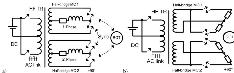
Fig.2. Circuit diagram of half-bridge converters system with a) central points of AC source; b) central points of motor loads
