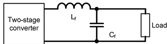
Fig.5. Connection of 2<sup>nd</sup> order LC filter between load and two-stage converter
