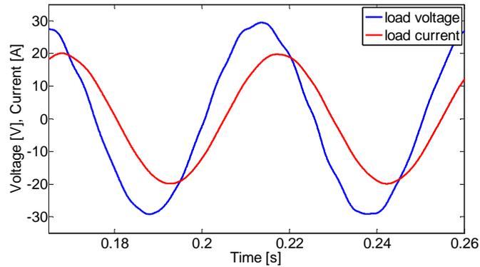
Fig.7. Matrix converter output voltage and current with LC filter with motor load (current waveform was fitted to the picture)
