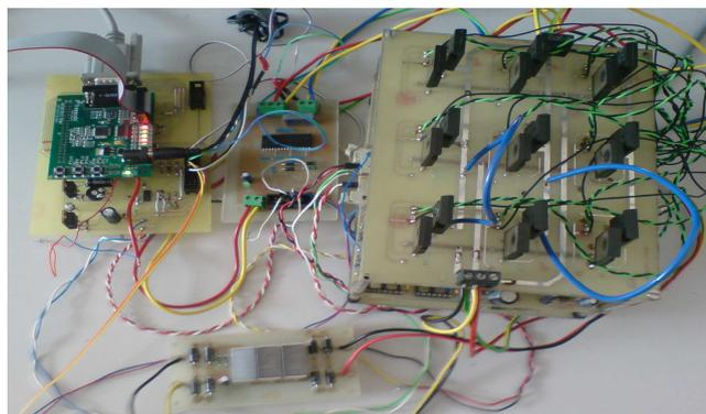
Fig.8. Physical model of two-stage converter
