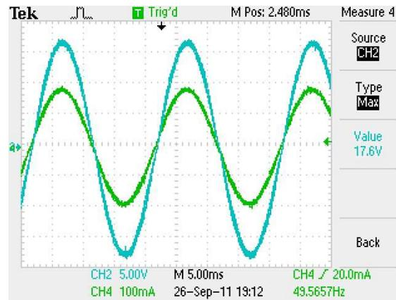
Fig.11. Output voltage (blue) and current (green) of two-stage converter with LC filter and resistive load
