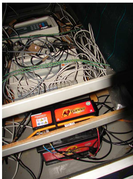
Rys. 2. Rejestratory KNE Data Logger z akumulatorem (12V)
