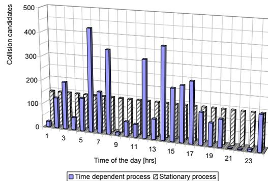
Fig.5. A number of collision candidates obtained from the MDTC model for constant and time varying traffic flows
