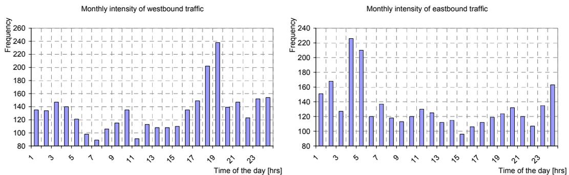
Fig.4. The marine traffic intensity of E-W flow, recorded between Helsinki and Tallinn
