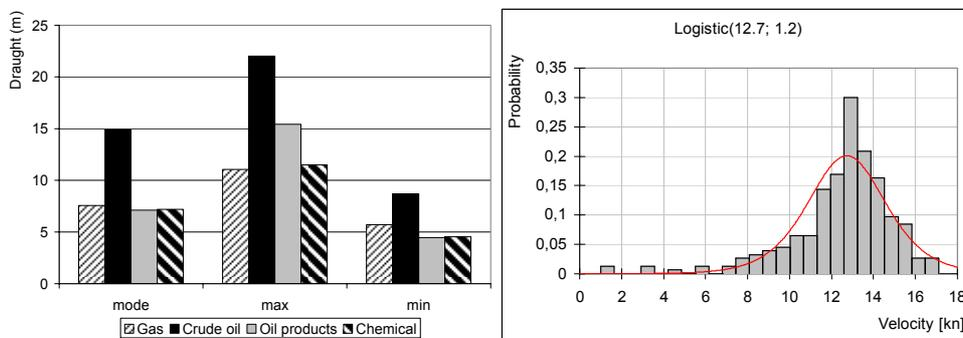
Fig.2. Distributions of the main parameters of tankers navigating in the Gulf of Finland
