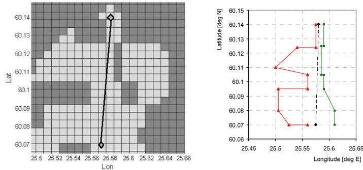
Fig.9. The safety contour obtained me means of gravity model (to left) and its generalization used for grounding probability calculation (right).
