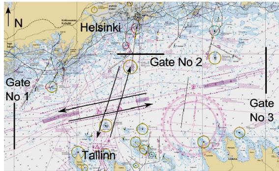
Fig.1. Analyzed waterways junction, with counting gates and main traffic flows [Montewka et al., 2010]
