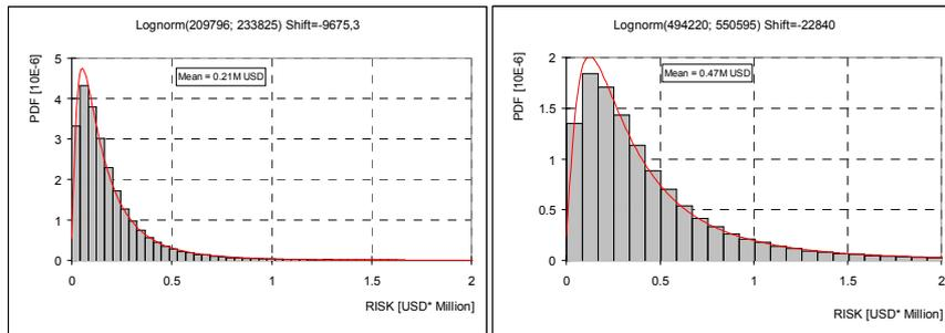
Fig.12. Distributions of random variable “RISK” in case of collision between a tanker and RoPax, for constant traffic intensity (left) and traffic intensity according to recorded data (right), summer traffic
