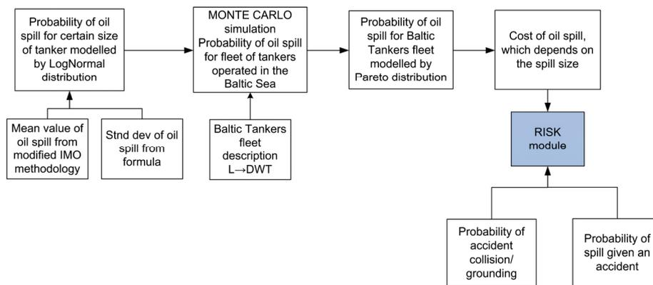
Fig.11. Block diagram of risk assessment process applied in presented study [Montewka, Krata, Kujala, 2010]
