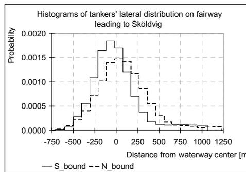
Fig.10. The overlaid two histograms of lateral distribution of tankers on the fairway to Sköldvik, a black dotted line represents north bound traffic whereas a solid black line is south bound traffic [Montewka, Krata&Kujala, 2010]
