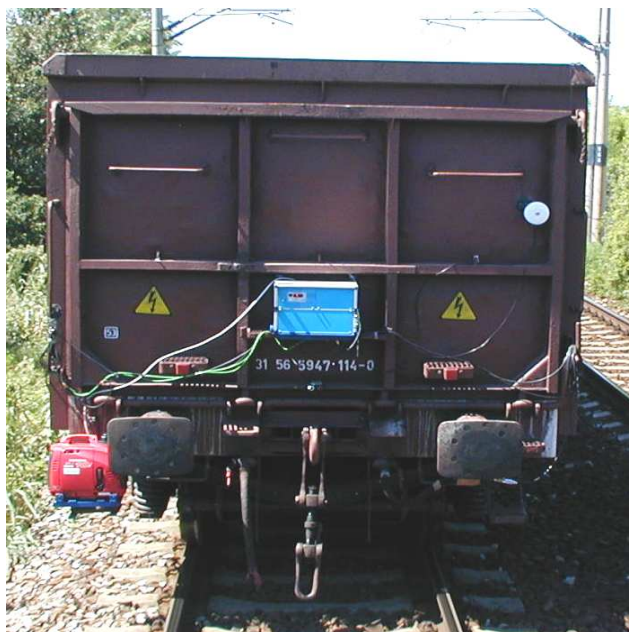
Fig. 3. Goods wagon Eas with a measuring device.
